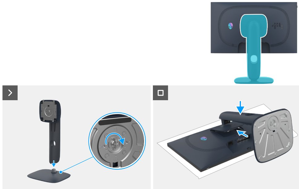
Figure 10. Installing the stand
