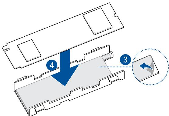
5. Remove the plastic film on the thermal pad on the heatsink cover.
