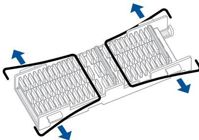
2. Lift and remove the heatsink cover.
