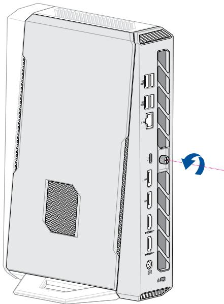
2. Push the main cover towards the rear of the system until it disengages from the system.
