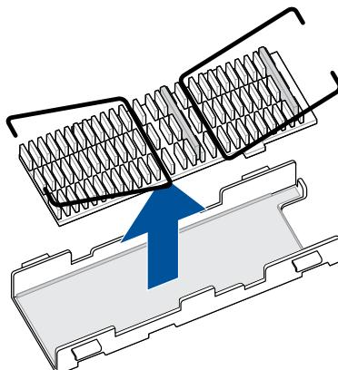
3. Remove the plastic film on the thermal pad on the casing of the M.2 2280 bracket.
