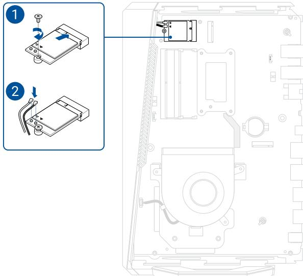
4. Place the wireless card shield over the M.2 module, and secure it using two (2) screws.
