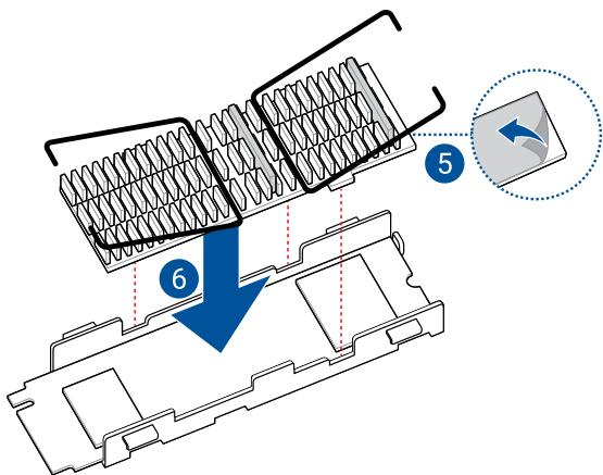
7. Push the wires into the hooks on both sides of the 2280 M.2 bracket to secure the heatsink cover.
