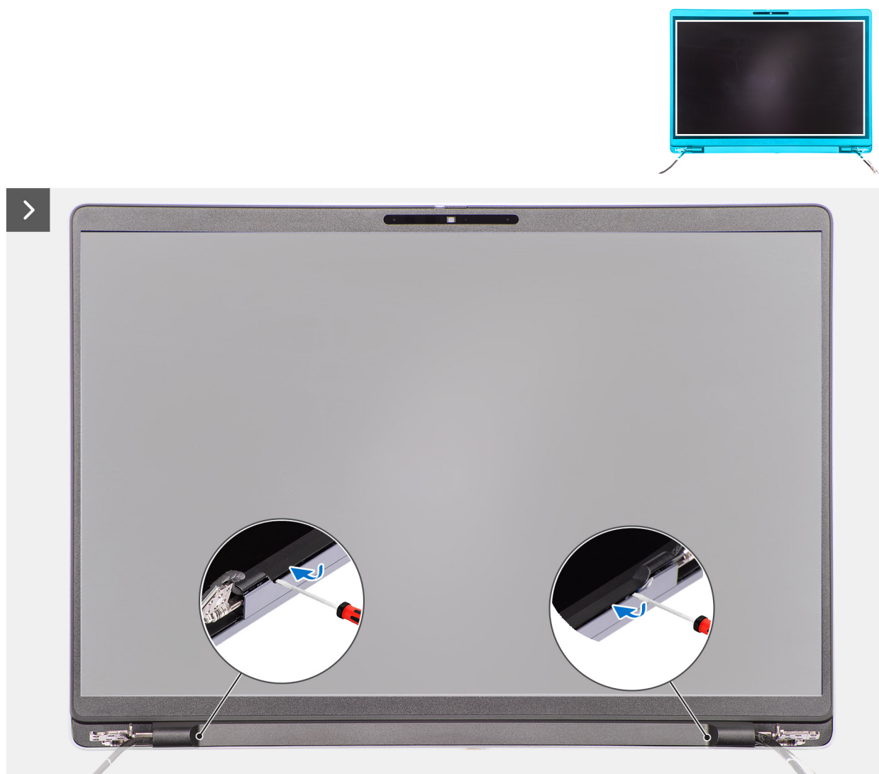
Figur 48. Removing the display bezel
