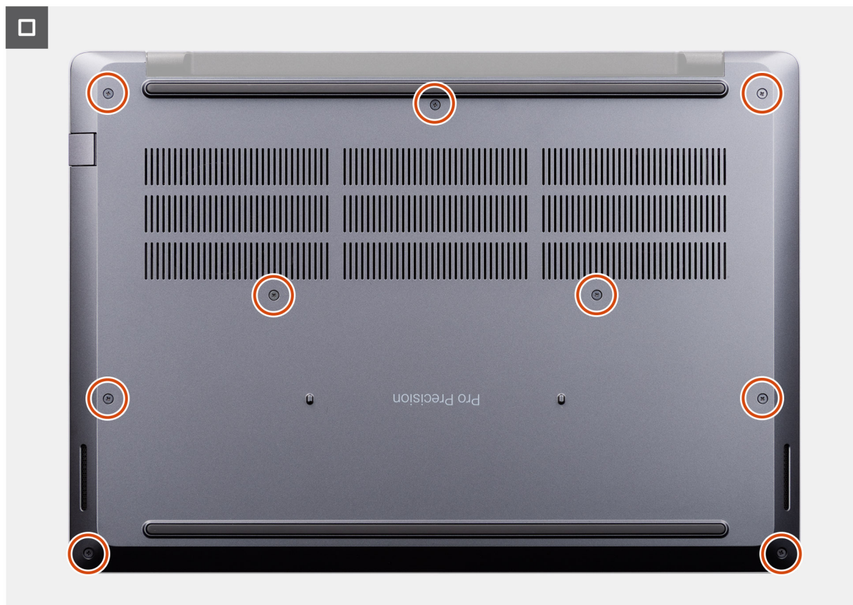
Figur 5. Installing the base cover
