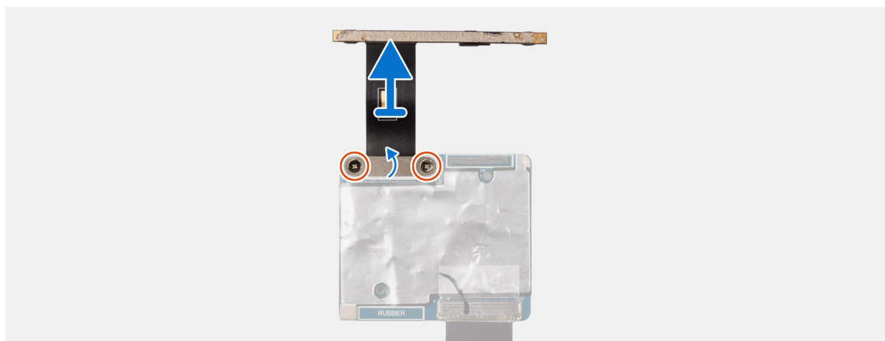
Figur 66. Removing the camera
