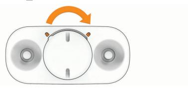
9 Insert the tool into the notches on the cover, and turn the cover clockwise.
