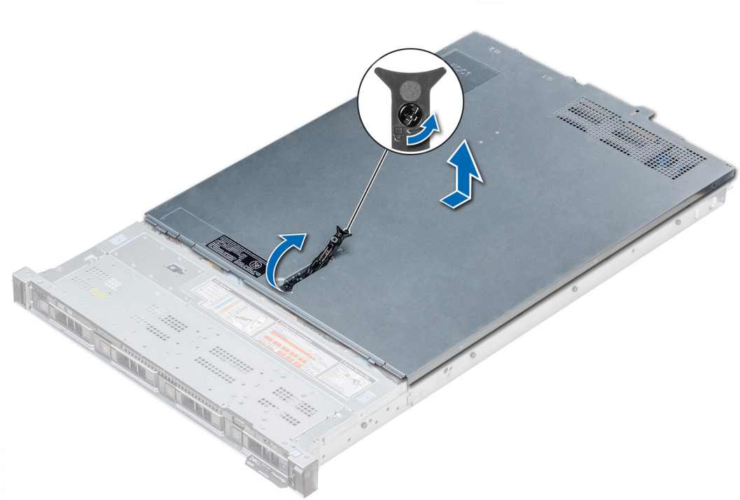
Figure 21. Removing the system cover
