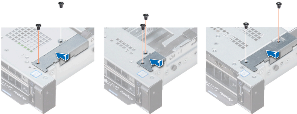
Figure 126. Installing the cable cover
