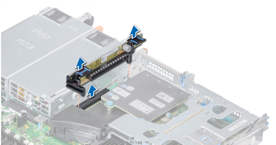
Figure 52. Removing the expansion riser 2A
