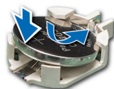
Figure 105. Installing the system battery
