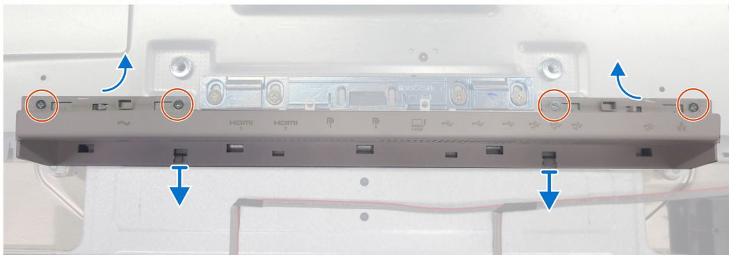
Figure 15. Removing the I/O cover
