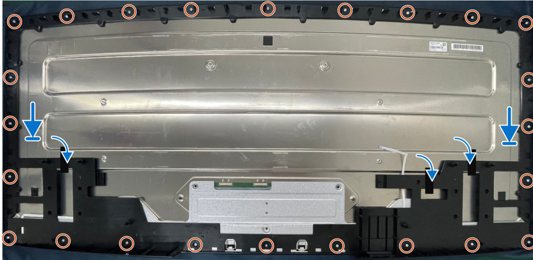
Figure 20. Installing the middle frame
