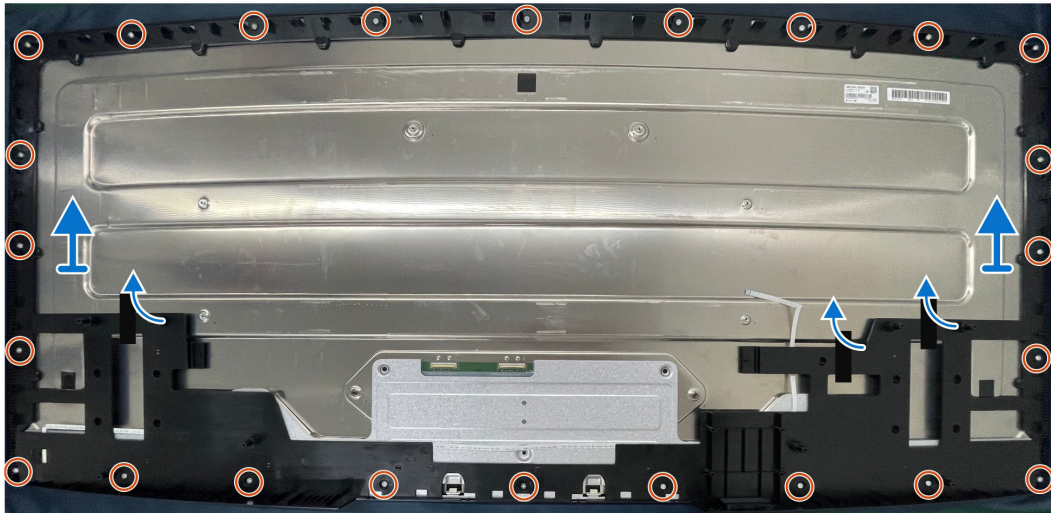
Figure 19. Removing the middle frame
