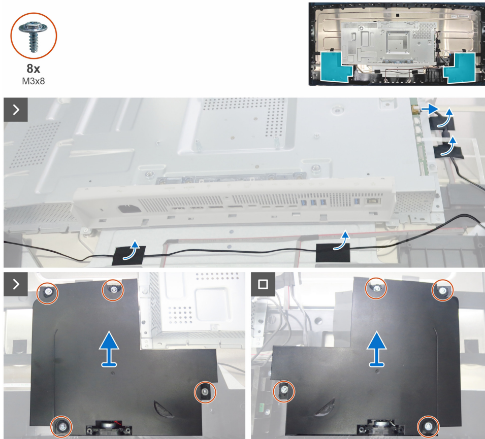
Figure 13. Removing the speakers
