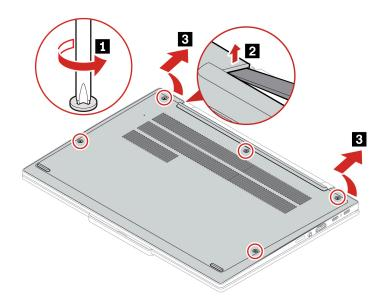
Step 2. Install the base cover assembly as shown below.
