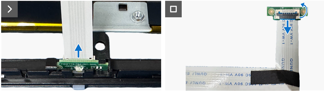
Figure 16. Removing the LED board
