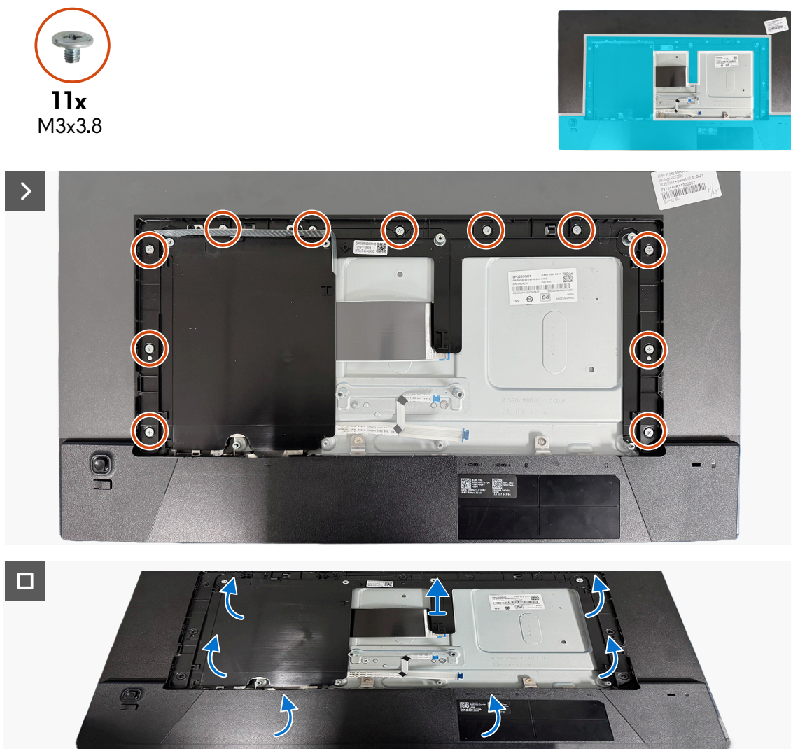
Figure 11. Removing the middle frame
