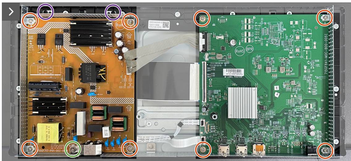
Figure 7. Removing the system board and power board
