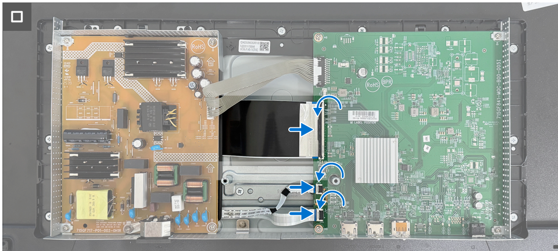
Figure 10. Installing the system board and power board
