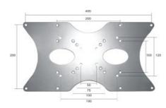
The NewStar VESA adapter, model FPMA-VESA400 allows a VESA mount with 50x50, 75x75, 100x100 and 200x100 mm interface to be used with displays with VESA hole patterns of 200x200mm, 400x200 and 120x180 mm (JVC holepattern). Ideal when flat screen needs different VESA pattern to select wall-, desk- or ceiling mount.
