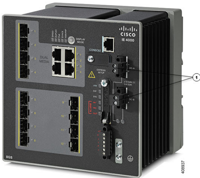
Figure 10 Removing the Power Connectors from the Switch
