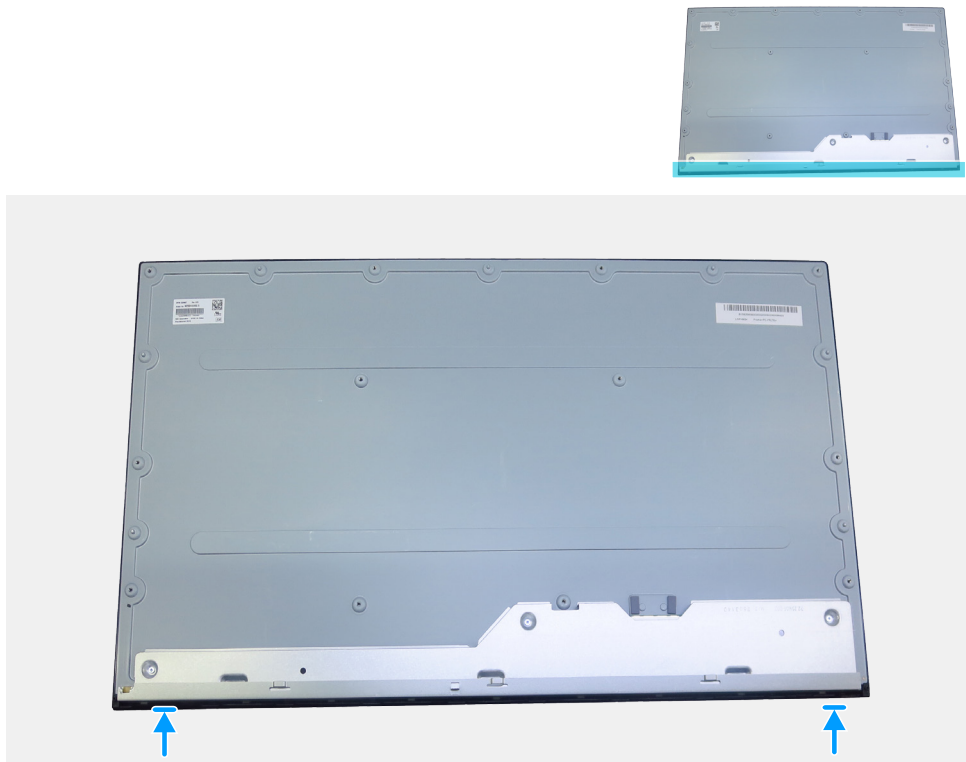
Figure 14. Installing the front bezel
