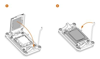
Make sure the CPU is aligned with the socket before locking it into place.
