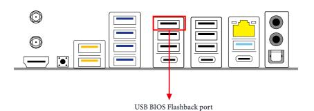
ASRock BIOS Flashback feature allows you to update BIOS without powering on the system, even without CPU.
