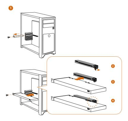
Skip Step 2 if you install a graphics card into PCIE1 slot. Illustrations here are examples only.
