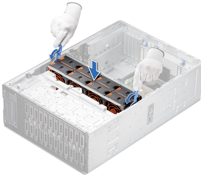
Figure 40. Installing the cooling fan cage
