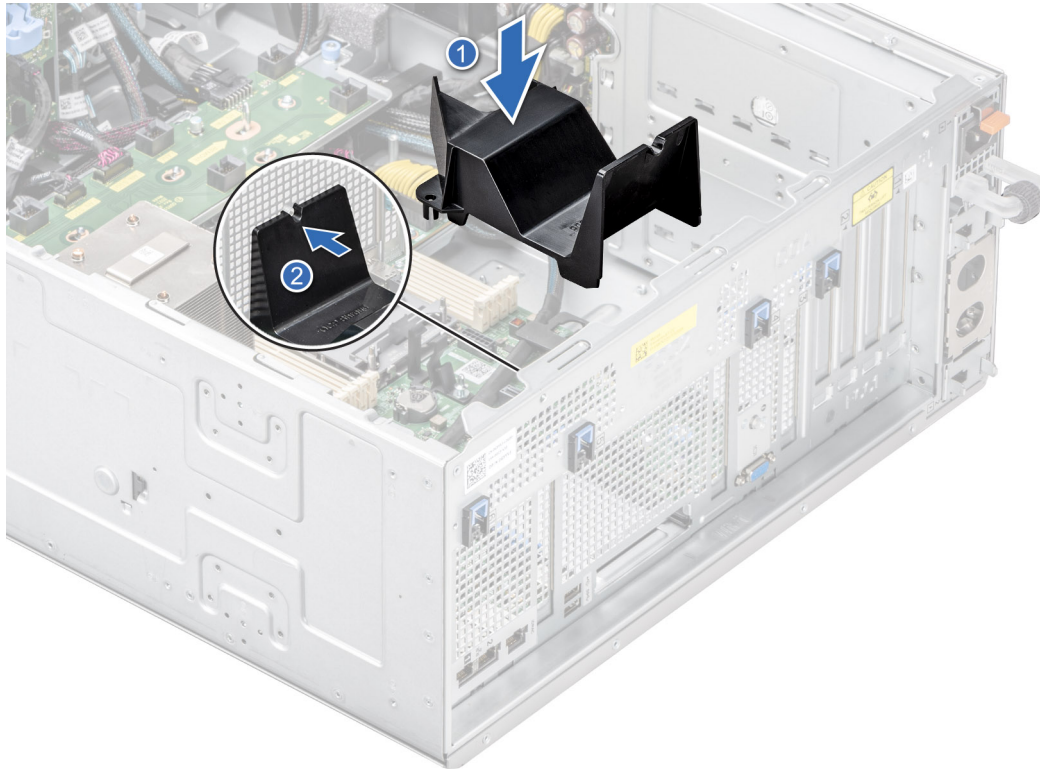
Figure 158. Installing the OCP air shroud.
