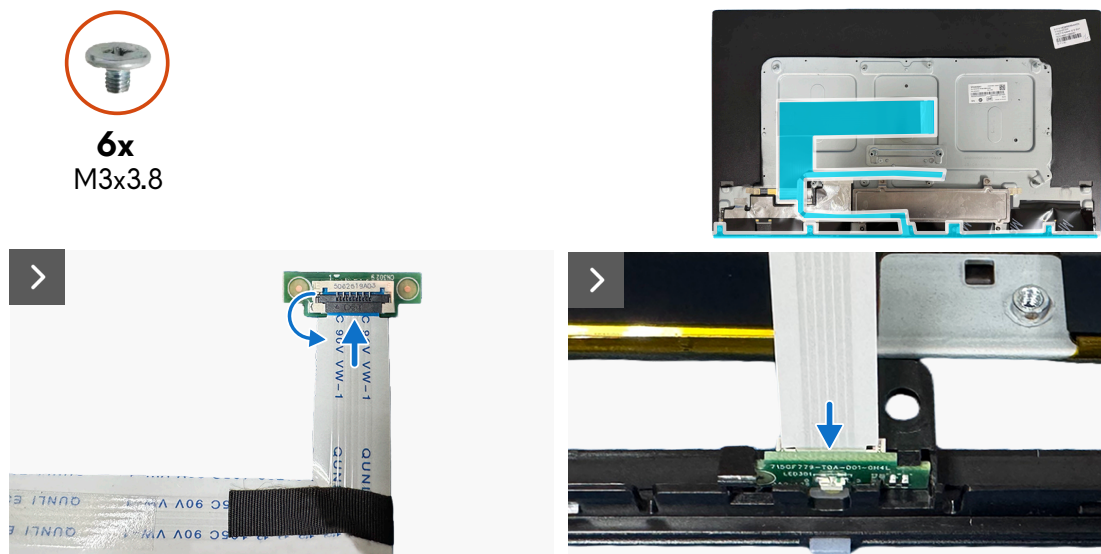
Figure 27. Installing the LED board
