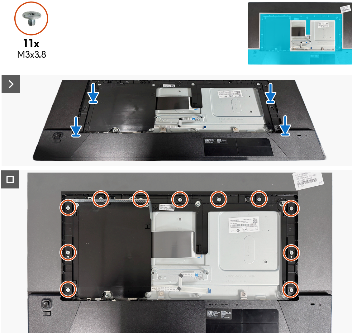
Figure 22. Installing the middle frame
