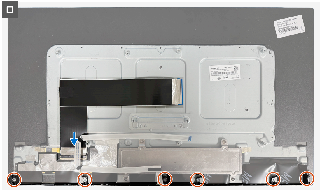
Figure 28. Installing the LED board
