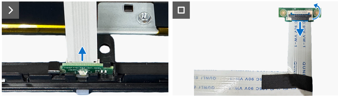
Figure 26. Removing the LED board
