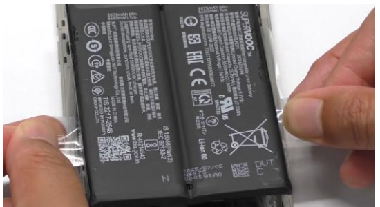
手机平放, 斜拉拉手贴, 缓缓斜拉让电池与易撕纸分离 Lay the phone flat, pull the battery handle diagonally, and pull the battery away from the battery pull tape slowly
