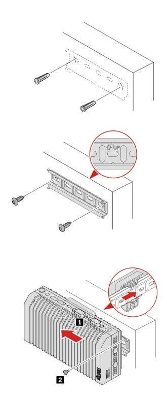
The replacement steps also apply to the computer with an IO expansion box installed. See "IO expansion box" on page 60.
