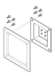
The NewStar VESA adapter, model FPMA-VESA100 allows a VESA mount with 75x75 mm interface to be used with displays with VESA hole patterns of 100x100. Ideal when flat screen needs different VESA pattern to select wall-, desk- or ceiling mount.
