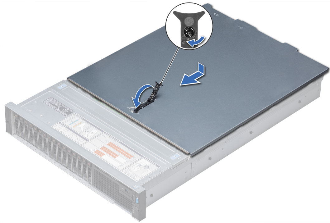
Figure 26. Installing system cover
