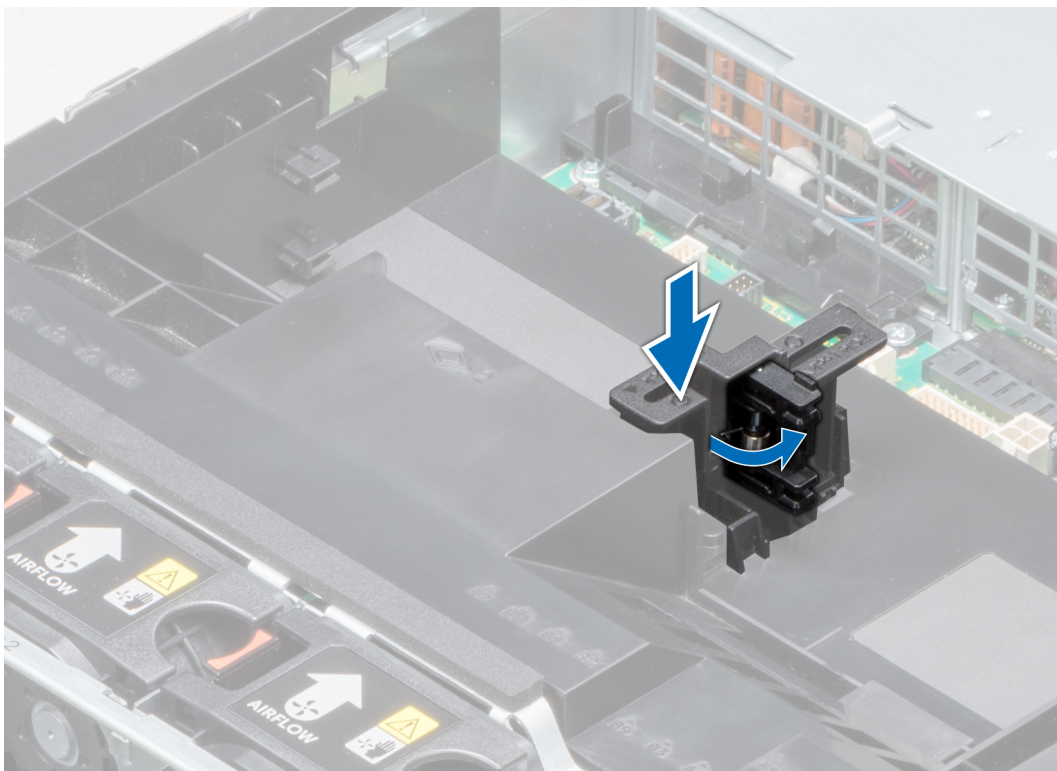
Figure 64. Opening the PCIe card holder latch
