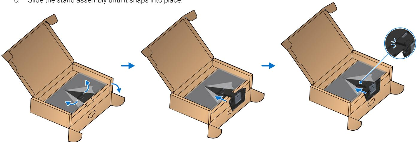
**Figure 11. Attach the stand assembly to the monitor**
