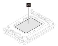
Figure 1. Illustrations of the thermal grease area
