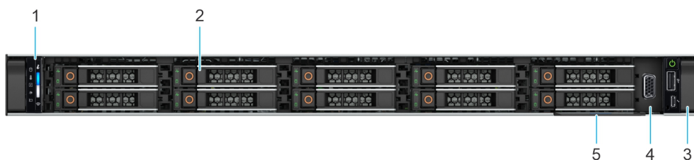
Figure 3. Front view of 10 x 2.5-inch drive system
