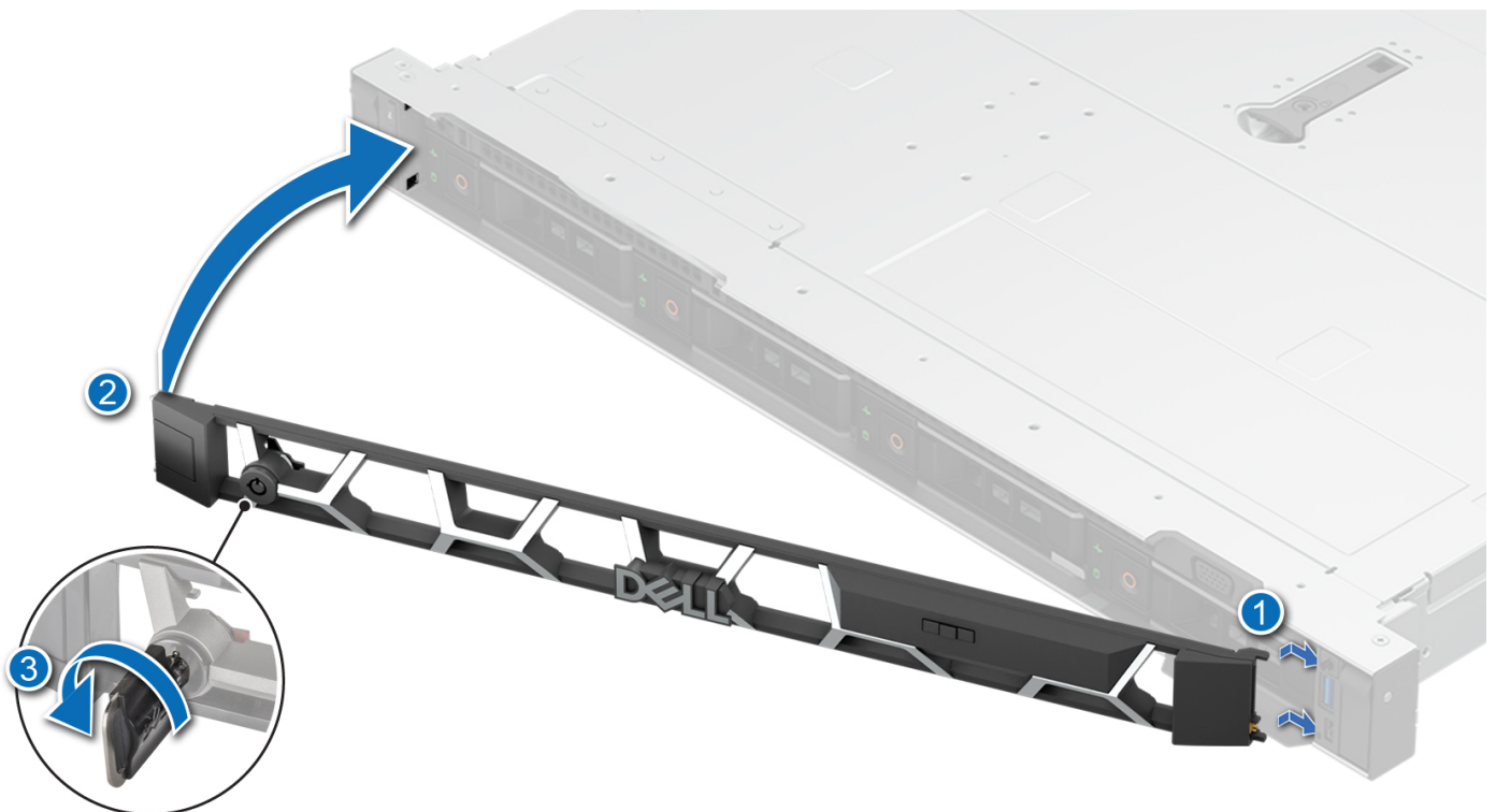
Figure 30. Installing the front bezel
