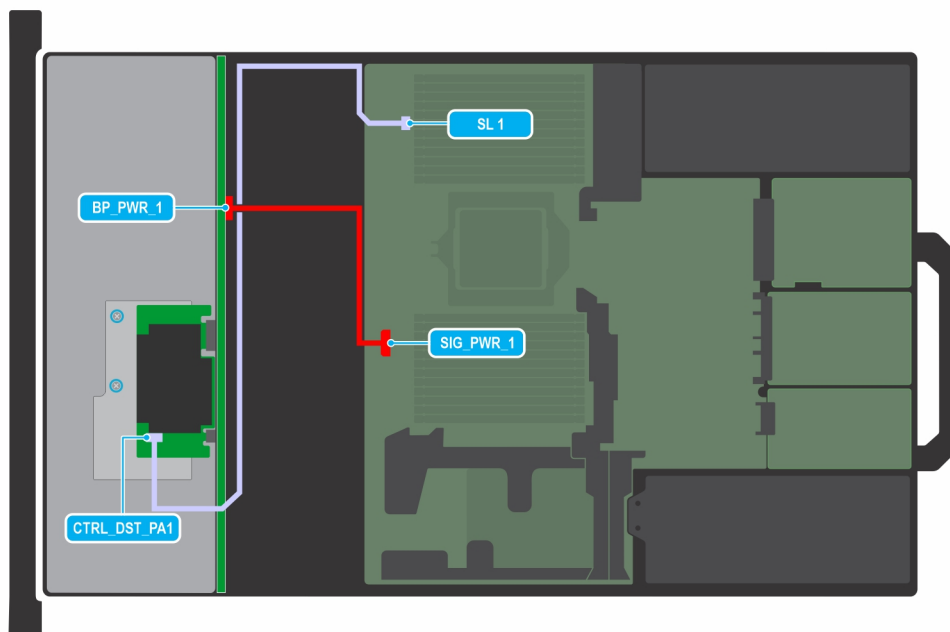
Figure 69. Configuration 1-1: 4 x 3.5-inch SAS3/SATA RAID
