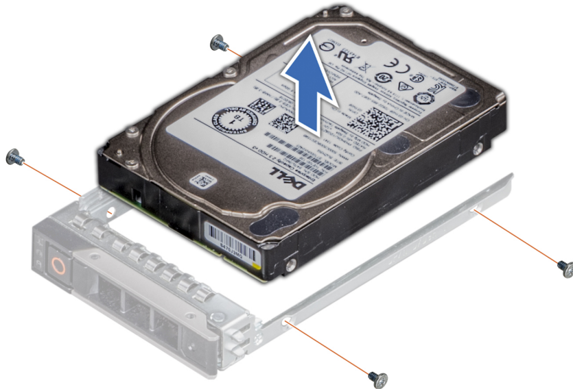
Figure 47. Removing the drive from the drive carrier
