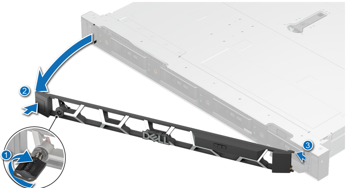
Figure 29. Removing the front bezel
