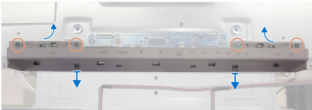
Figure 29. Removing the I/O cover
