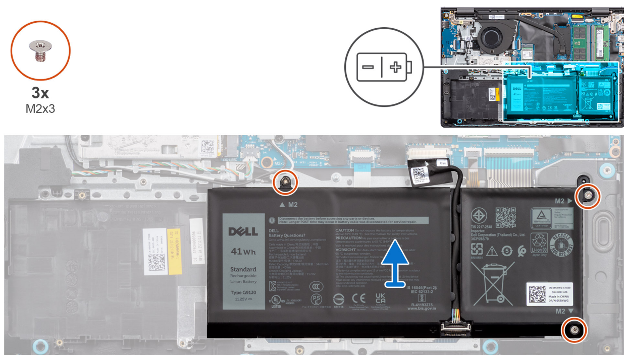
Figur 8. Ta bort 3-cellsbatteriet
