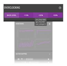
The overclocking feature included in Pi Tool modifies the following values in /boot/config.txt: over\_voltage, arm\_freq, gpu\_freq.
