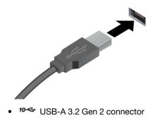
Charge USB-A compatible devices with the output voltage and current of 5 V dc and 0.9 A.
