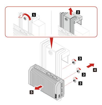
**Note:** When installing the Z hook kit, fasten the screws correctly to ensure that the computer is stable.
