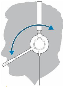
CAUTION: To avoid breaking the boom, only rotate it up and over 180°.
